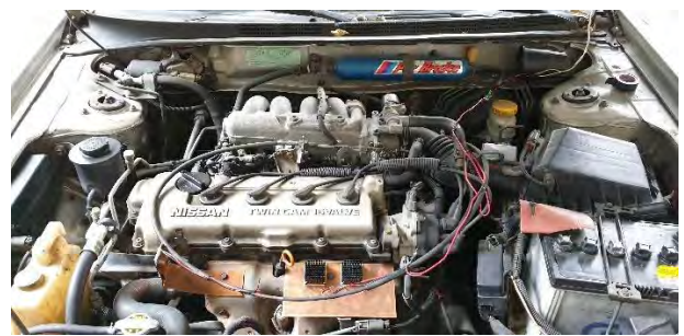
溫差晶片通過升壓晶片接線至車內
