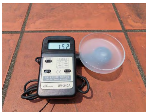
圖30 凝膠含培養皿遮蔽時紫外線強度:1520 \mu\text{W}/\text{cm}^2
