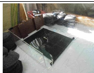
貼上砂紙的壓克力板斜坡能模擬傾斜沙灘
