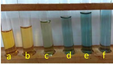
圖：200ppm碘液不同毫升加入5% 硼酸水溶液分別為a = 0 ml，b = 1ml，c = 2 ml，d = 3 ml，e = 4 ml，f = 5 ml
