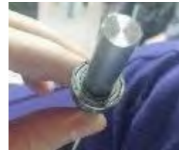
圖4-16 內徑10mm外徑19mm之軸承
